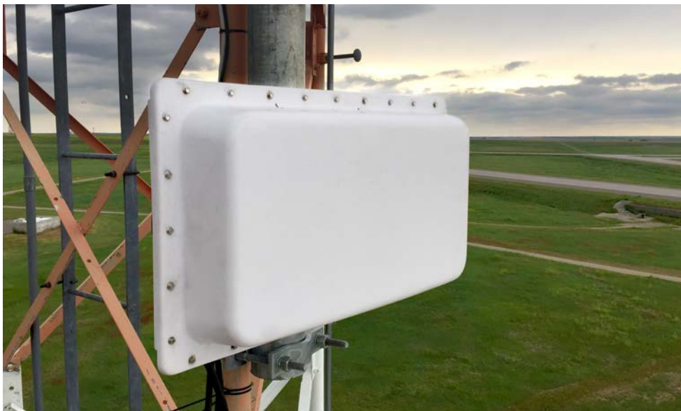
A GroundAware security array can provide security up to 2,000 acres
